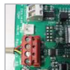
Figure 3. AquaLink RS 485 Communication (4-Wire Connection)
